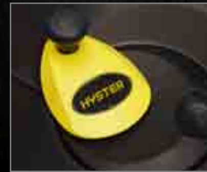
Steer tiller handle position is operator adjustable (Opt. on ZRS 2 ) and steer effort is adjustable to reduce operator fatigue.
