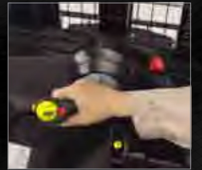
Optional Side stance control is configured with the operator in mind and offers simultaneous control of travel and hydraulic functions.
