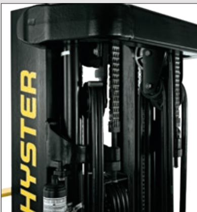
Free-floating lift cylinders further extend rod and seal life.
