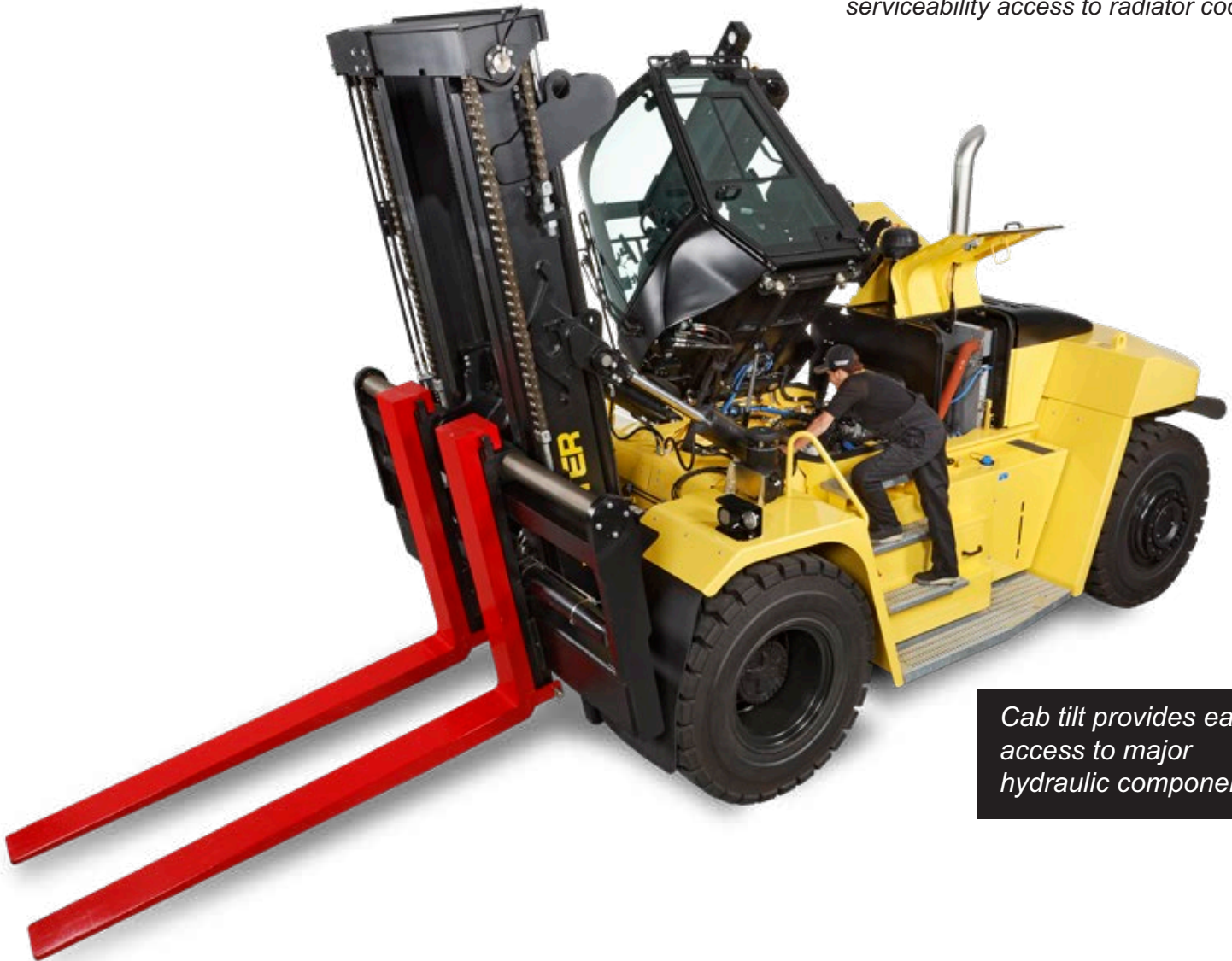
Hinged cover enables easy serviceability access to radiator cooler
