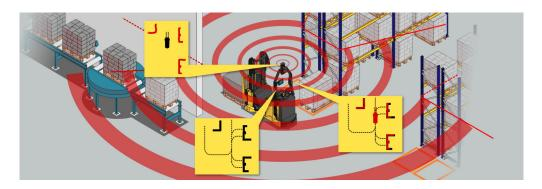
To understand their location while in operation, mobile robotics use LiDAR to get the real-time "view" of surroundings
