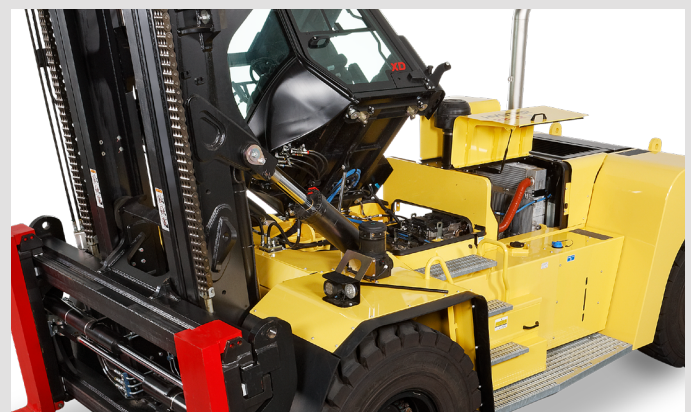
Optional powered cab tilt provides easy access to major hydraulic components
