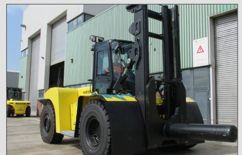
Apron-style sideshift with individual hydraulic fork positioning
