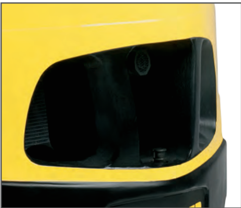
Counterweight tunnel design improves airflow
