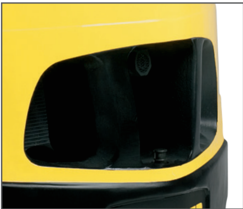
Counterweight tunnel design improves airflow
